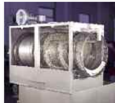
Rotary drum washer barrel with panels removed.
