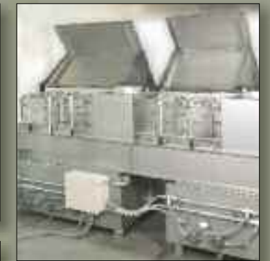
Stainless steel wash and rinse section hoods to show spray manifolds.
