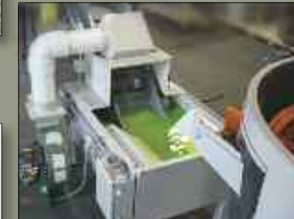
Anti-rust drag-out conveyor system complete with heaters and moisture blow-off. Features 12" wide belt and 85 gallon inhibiting tank.
