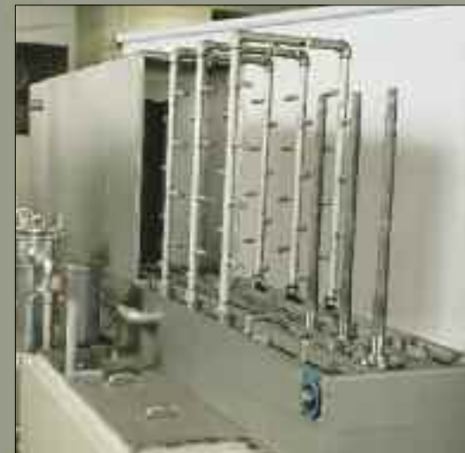
Heightened spray manifold for long parts.
